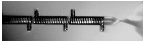
Fig. 1. A micro machined nozzle with 3 heater coils positioned just before the nozzle throat. The nozzle throat is approximately 30 μm in a heat exchange chamber.
